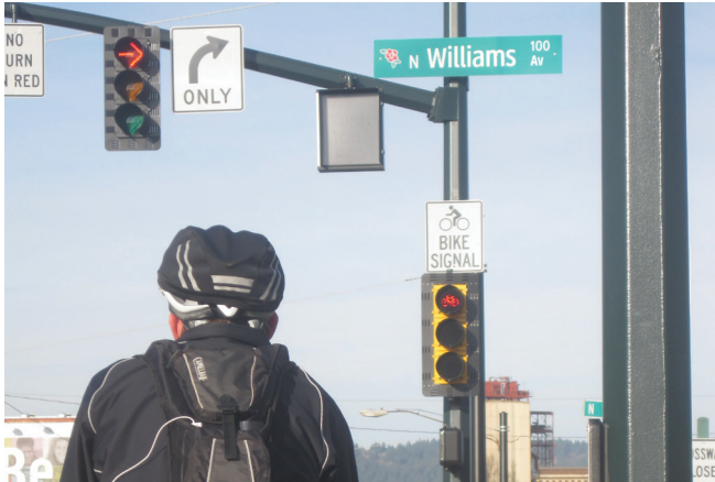
Figure C2. Bicycle Signals should be considered to create safe interactions at right-turn only lanes.
