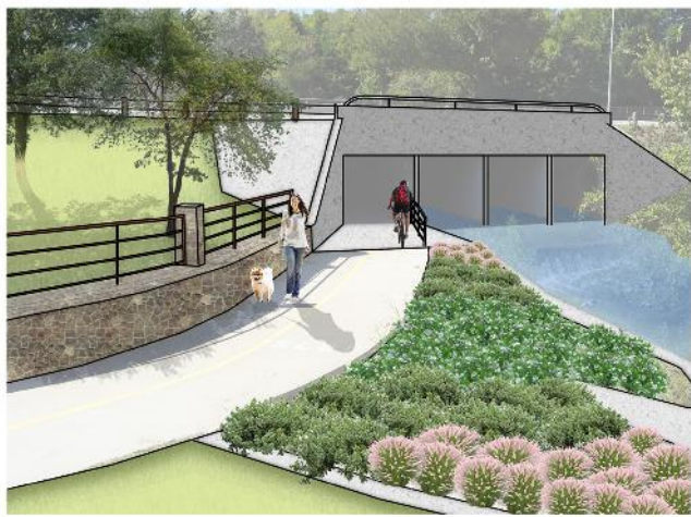
Figure 9: Typical Trail Culvert Underpass
